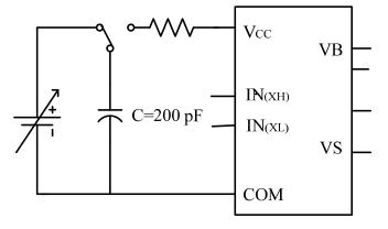
Figure 5-6. ESD Test Circuit (insides IC)
