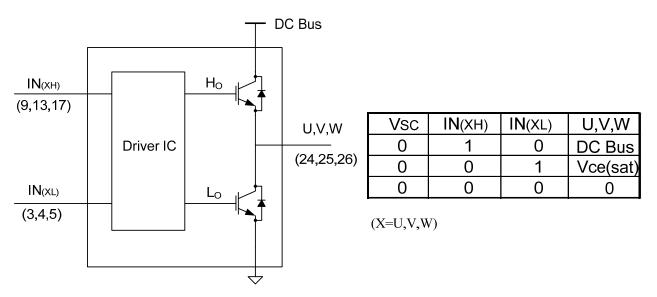
Figure 4-11. Input/Output Signal Circuit
