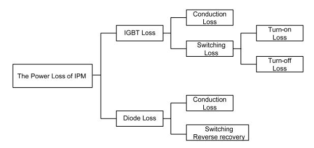
In order to obtain the accurate switching loss, we should consider the DC-link voltage of the IPM system, the applied switching frequency and the power circuit layout in addition to the current and temperature. In this chapter, use these power loss calculations in order to design enough cooling to keep the junction temperature  $T_j$  below maximum rated value. Therefore two most important sources of power dissipation that must be considered are conduction losses and switching losses.
