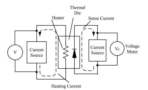
Fig. 7-4 Illustration of Thermal Test Die Test Method Concept
