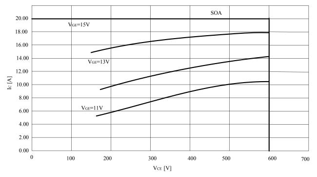
Figure 5-4. Safe Operating Area During Short-Circuit (SCSOA)
