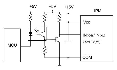
Figure 4-2. Interface Circuit Between ID-IPM and MCU
