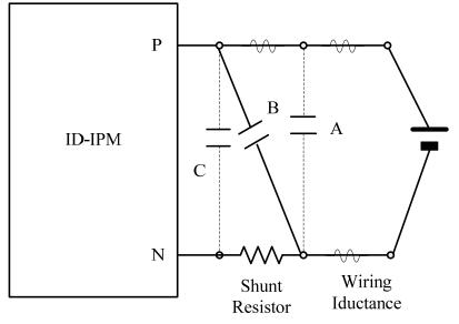
Figure 4-18. Recommended snubber circuit location
