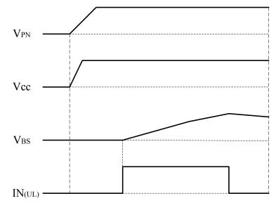
Figure 4-5. Timing Chart of Initial Bootstrap Operation Charging
