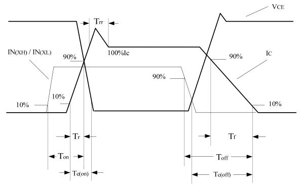
Figure 2-2. Definition of Switching Time
