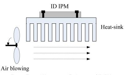
Fig. 7-7 Thermal Measurement Environment of ID-IPM
