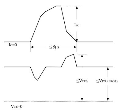
Figure 5-2. SOA for Short-circuit
