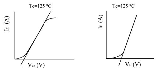
Figure 8-2 Output Characteristics of IGBT and Diode
