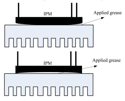
Figure 3-6. Heat Sink Flatness Specification
