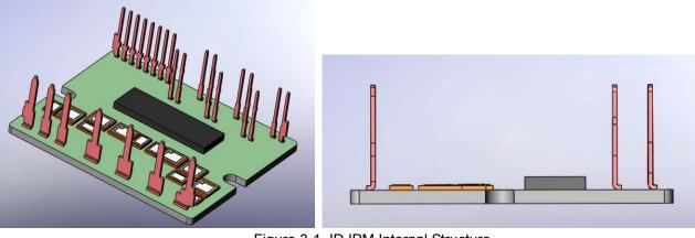
Figure 3-1. ID IPM Internal Structure
