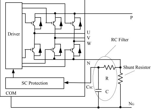
Figure 4-15. Example of External RC Filter Circuit
