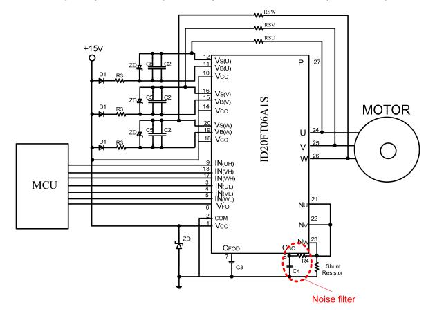
Figure 9-2. Noise Filter Circuit
