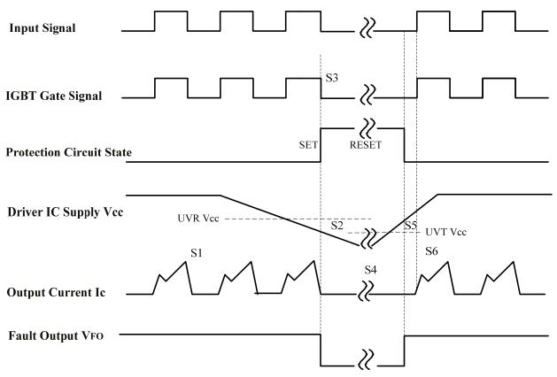
Figure 4-13. Timing Chart of Under-Voltage Operation
