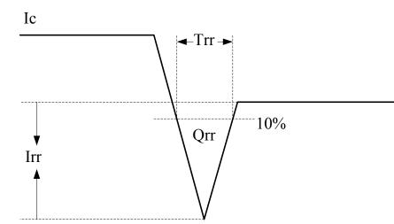
Figure 8-3 Diode loss
