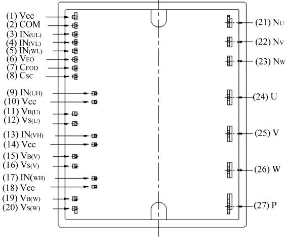
Figure 2-1. Pin Definition of ID IPM (ID20FT06A1S)
