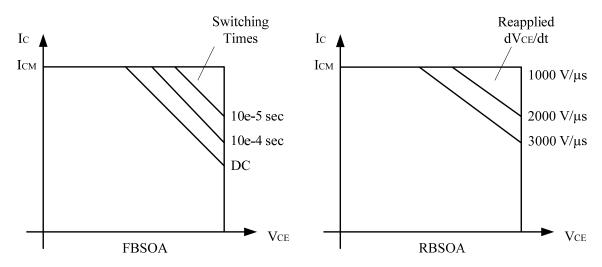
Figure 5-3. Safe Operating Area During Switching
