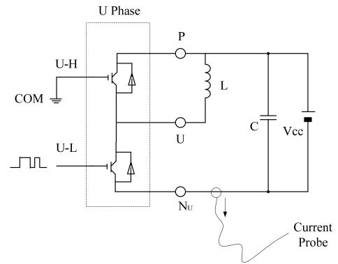
Figure 2-4. Test Circuit of Dynamic Parameter
