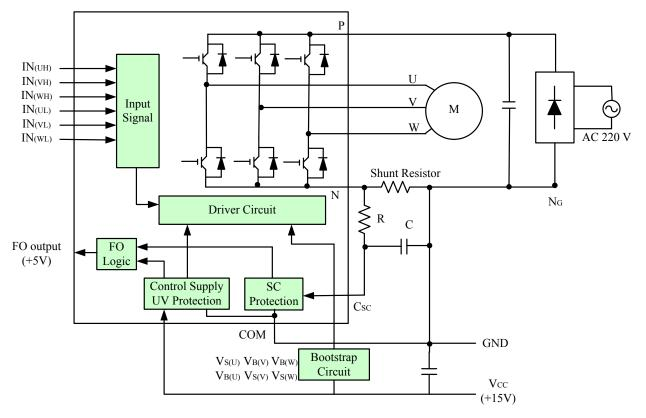
Figure 4-1. System Block Diagram of the IPM
