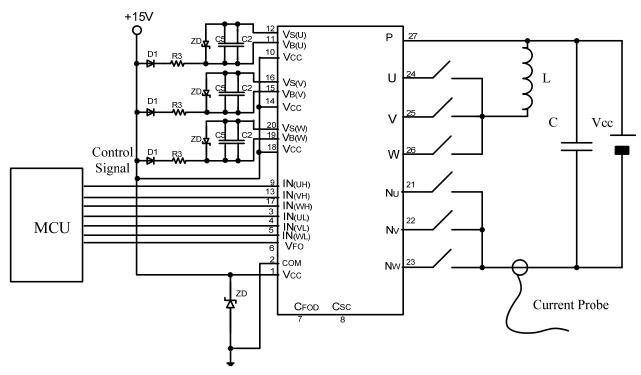
Figure 2-3. Evaluation Circuit Diagram (Inductive Load)
