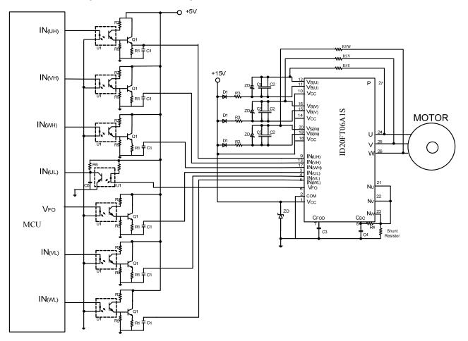
Figure 4-9. Typical Application Circuit Interface Example with Photo-Coupler
