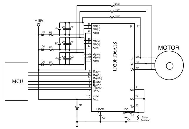
Figure 4-8. Typical Application Circuit Interface Example with Direct Input (Without Photo-Coupler)
