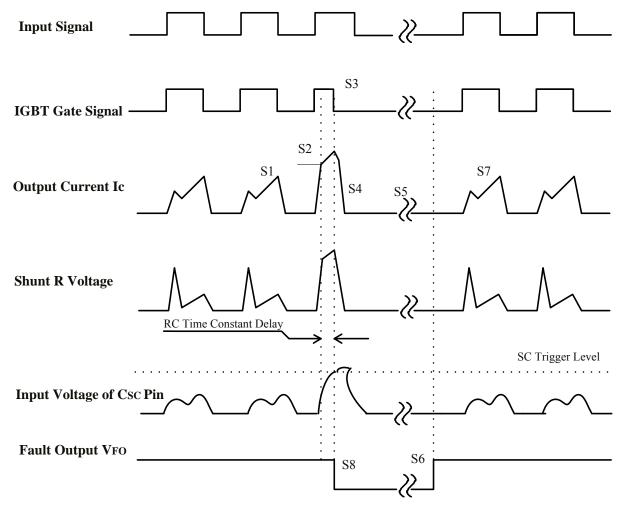
Figure 4-12. Timing Chart of SC Operation
