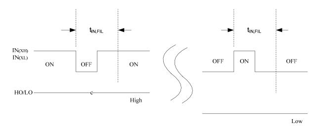
Figure 4-21. Input Filter Function
