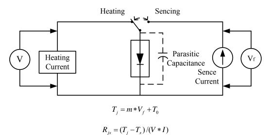
Fig. 7-6 Illustration of Diode Test Method Concept
