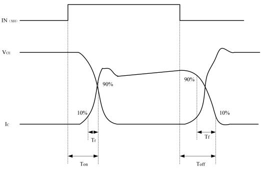
Figure 2-5. Switching Time Definition
