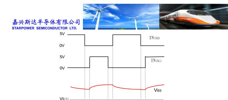
Figure 4-7. Charging and Discharging Action of the Bootstrap Capacitor Timing Chart
