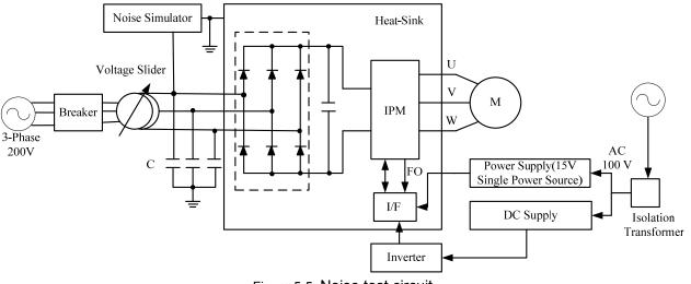
Figure 5-5. Noise test circuit
