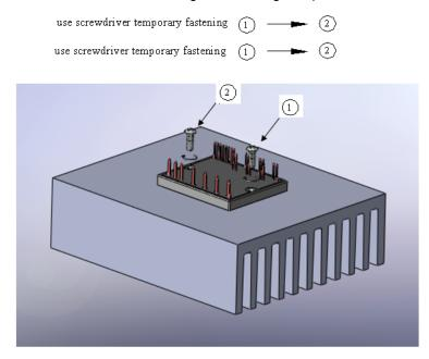
Figure 3-5. Recommended Fastening Order of Mounting Screws
