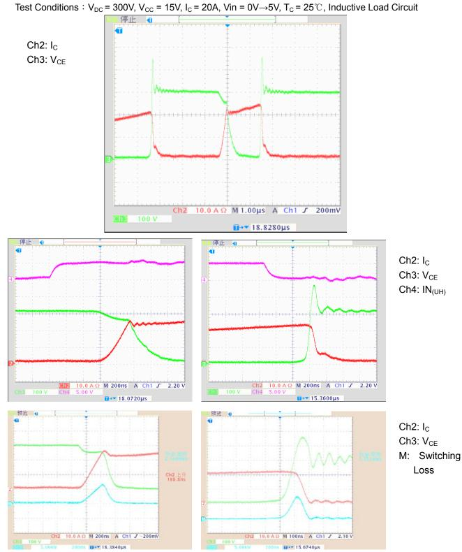
Figure 2-6. Switching Waveform of ID- IPM (Used ID20FT06A1S class) (Typ.)
