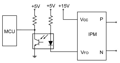
Figure 4-14. Diagram of FO pin Measurement Circuit
