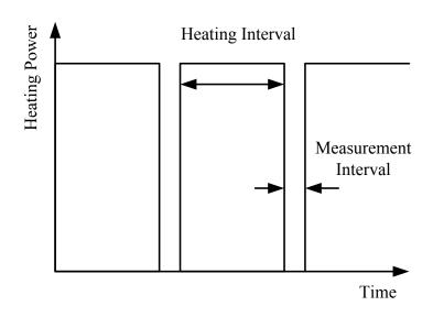
Fig. 7-5 Graphic of Illustration of the Heating and Measurement Intervals
