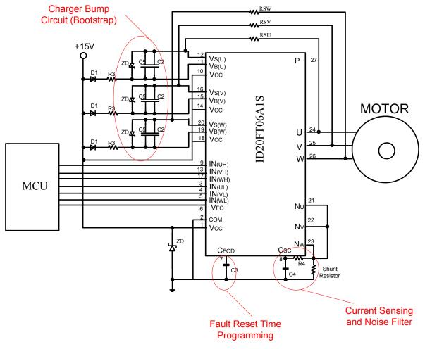
Figure 9-1. Application Circuit
