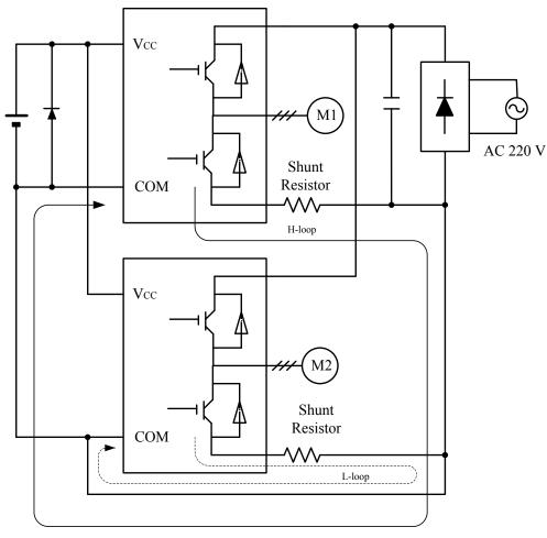
Figure 4-20. Parallel Connection
