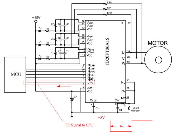
Figure 9-3. FO Signal Circuit
