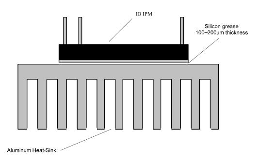
Figure 3-3. Recommended Silicon Grease Thickness
