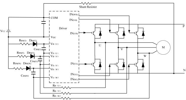
Figure 4-6. Inverter Circuit Diagram
