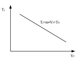
Figure 7-3. Typical Example of a TSP Plot with Constant Sense Current
